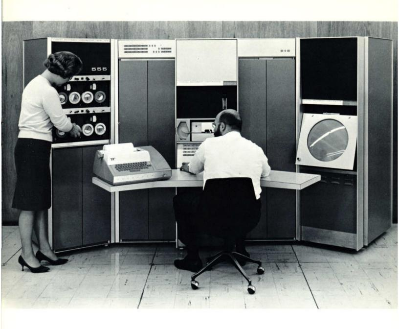
The basic PDP-7 can be easily expanded using the many standard options available. Shown in the above configuration are DECtape transports and control unit along with a high speed graphic and character display Type 340 (2 right-hand cabinets). Such a
