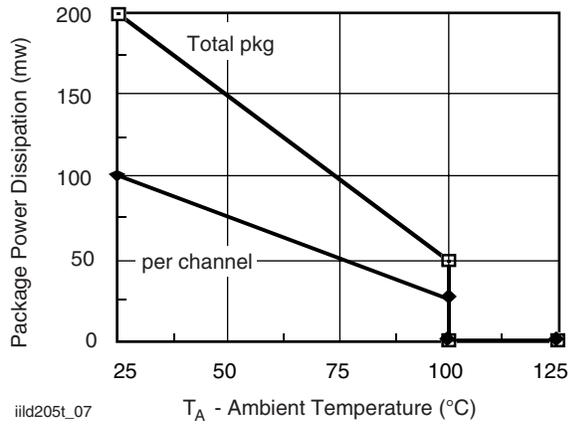
Fig. 7 - Power Dissipation vs. Ambient Temperature
